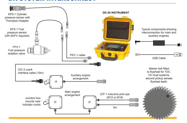
The Doctor instrument is available in two versions, namely the single channel DK-20 for cylinder pressure only measurements, and the two channel DK-20/FV which incorporates a second channel for simultaneous fuel or vibration measurement.
